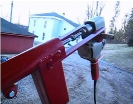
**Low speed drill attached to auger to lift pellets**
